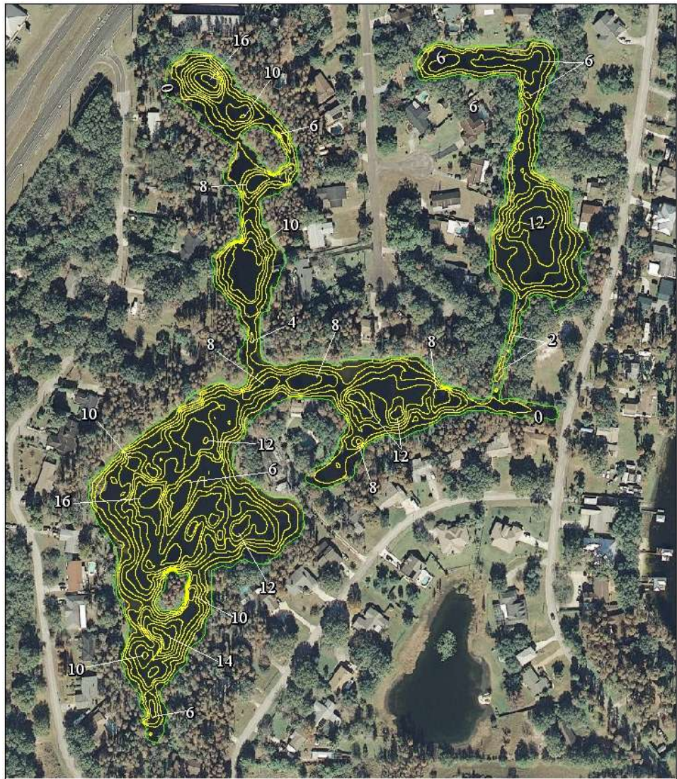
Figure 2. 2011 2-Foot Bathymetric Contour Map for Little Lake Wilson
