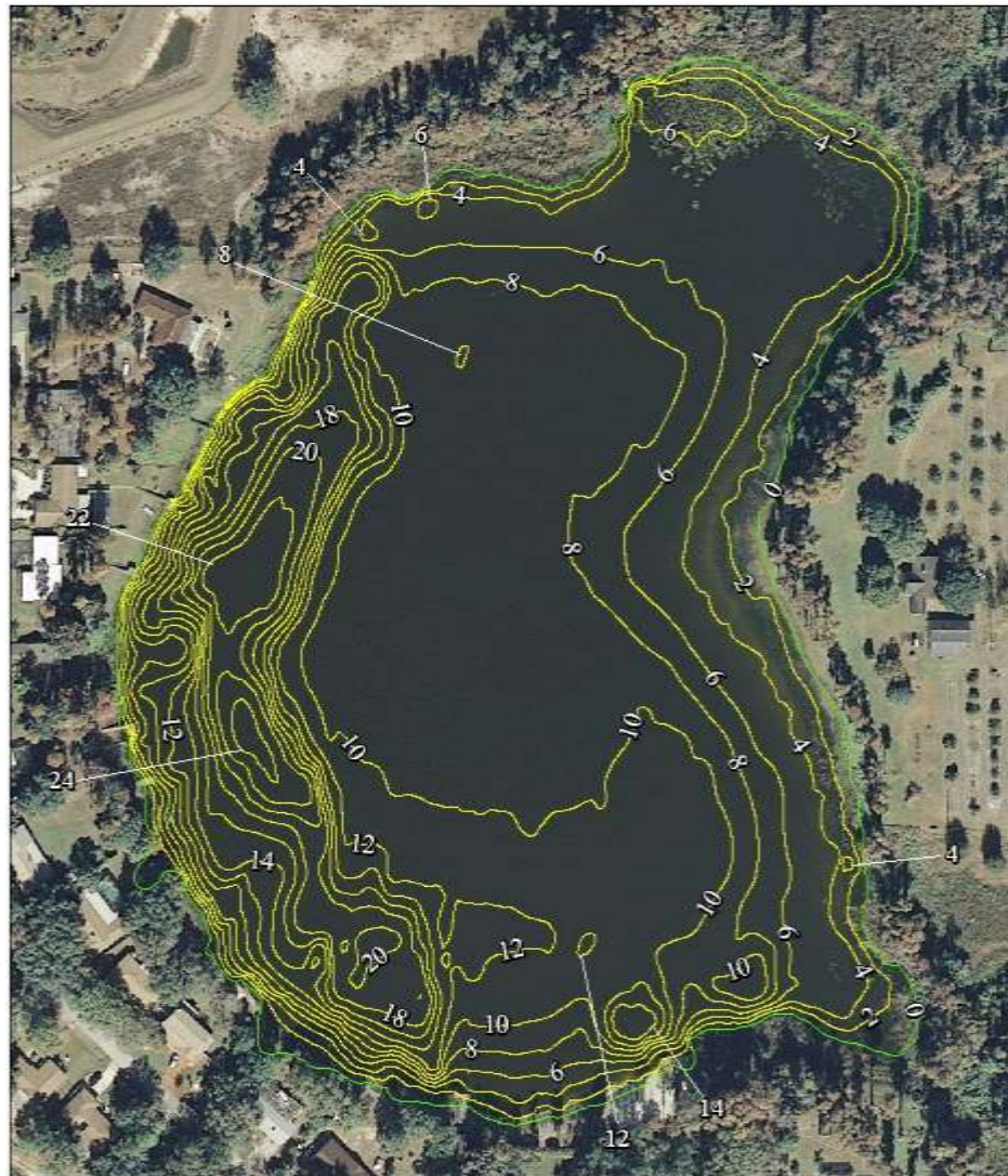
Figure 2. 2011 2-Foot Bathymetric Contour Map for Lake Harvey
