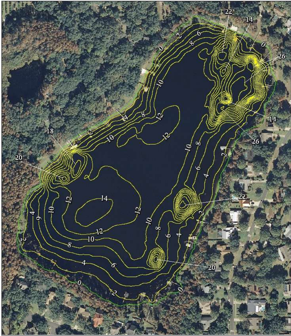
Figure 2. 2011 2-Foot Bathymetric Contour Map for Lake Armistead
