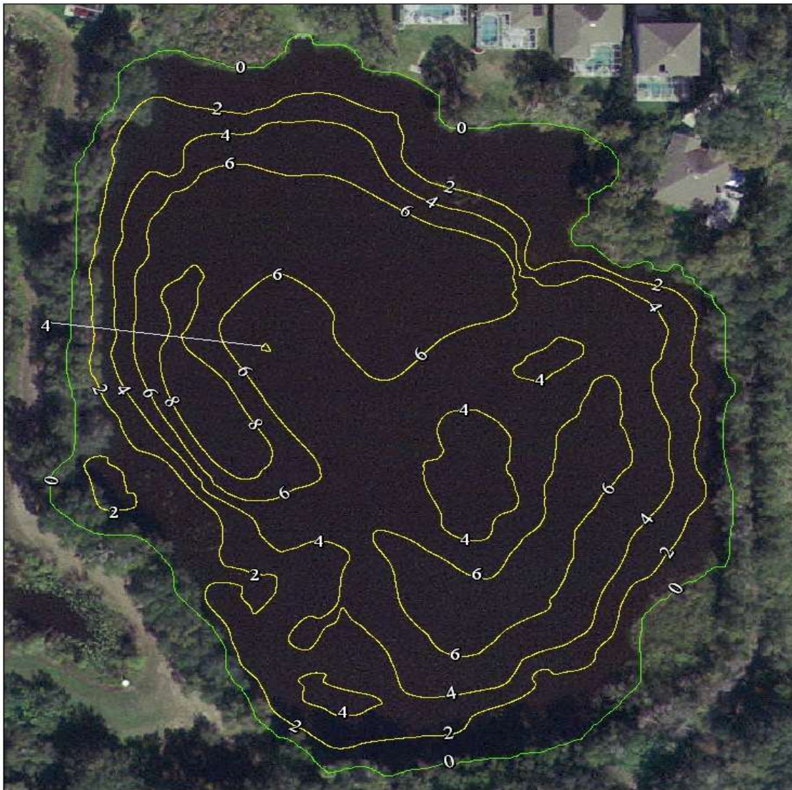
Figure 1. Contour map for June Lake. The mapping technique used in 2009 employs a standard DGPS for horizontal position and a fathometer for depth.
