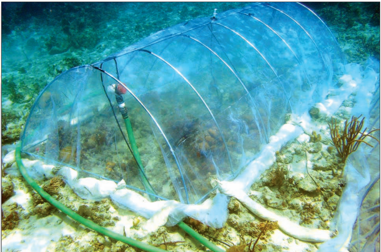
This underwater respirometry device (photo not taken in the preserve) is one of the innovative approaches to studying ecosystem function in the USGS Tampa Bay Study. Photo courtesy of USGS.
