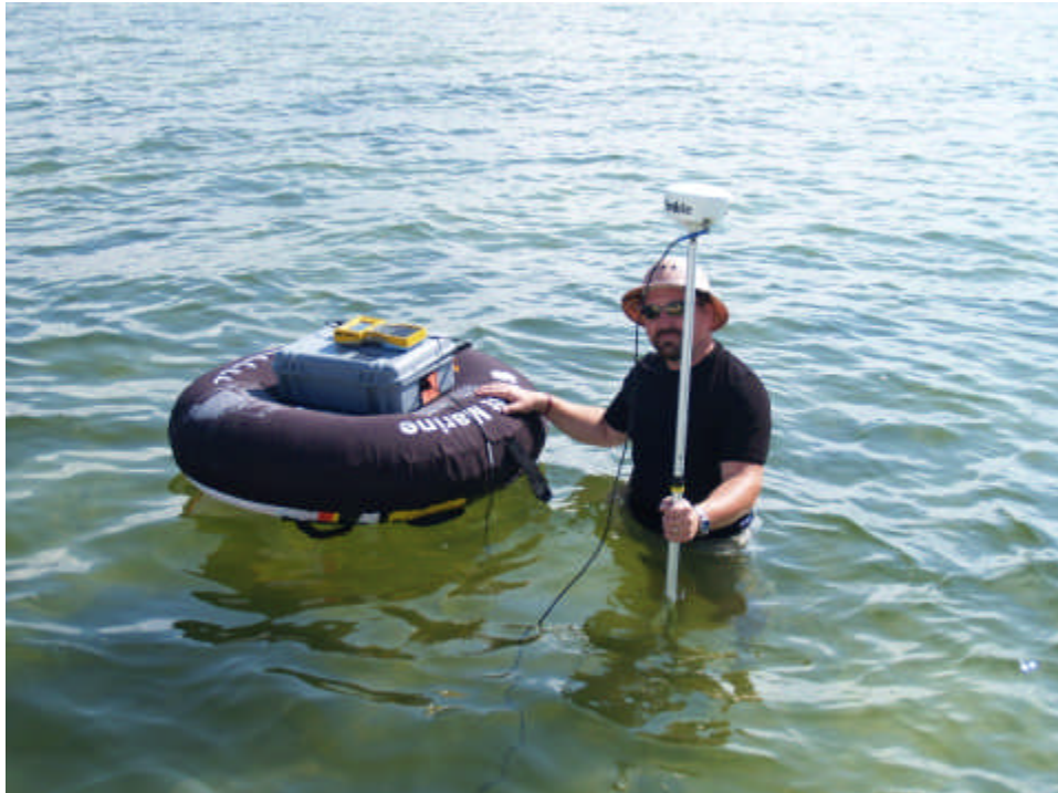
Figure 11. Method used to obtain GPS coordinates of donor plug sites.
