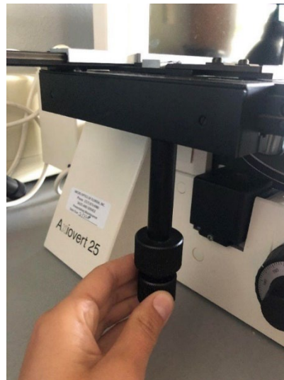
Figure 6. Photo showing the stage directional wand.
