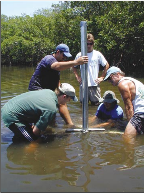
Retrieving a sediment core from Tampa Bay.
