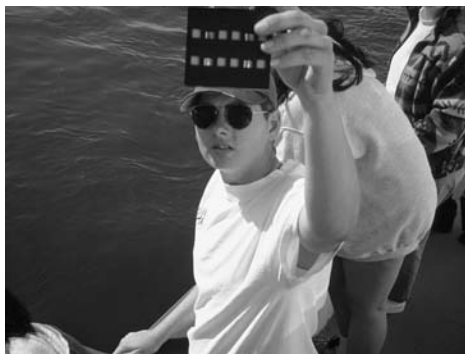
Many field test kits require the monitor to compare the colors of a prepared water sample with a standard (photo by K. Register).
