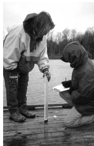
Using a transparency tube is an easy way to measure the water transparency. It is especially useful in water that is too shallow for a Secchi disk (photo by K. Register).
