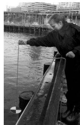
A volunteer takes a Secchi disk reading from Puget Sound (photo by E. Ely).
