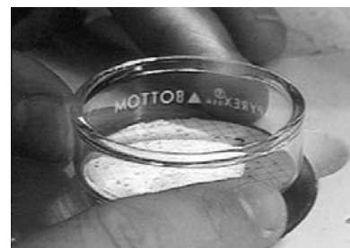
After incubation, any fecal coliform bacteria in the water sample will have grown into a colony (when using mFC medium or broth). These are called colony forming units (cfu) (photo by University of Maine Cooperative Extension).
